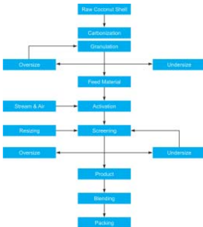
Flowchart of activated carbon manufacturing process
