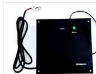
Acoustics based red palm weevil detector
