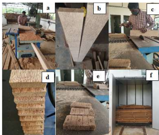
Fig.7(a) Planing, (b) Planed samples, (c) Sampling, (d) samples for QDT, (e) samples for physical property measurements, and (f) Kiln drying
